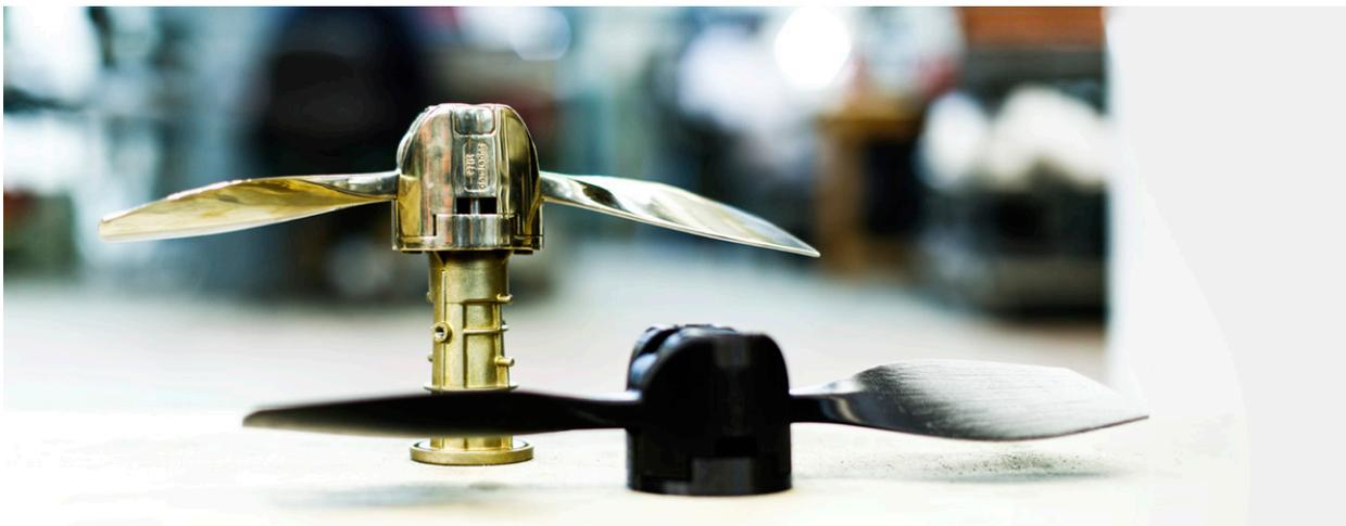
British manufacturing company Sylatech uses 3D printing to verify that pre-production items are dimensionally accurate and function as intended. When design requirements are met, these items are used to manufacture metal parts through investment casting.
