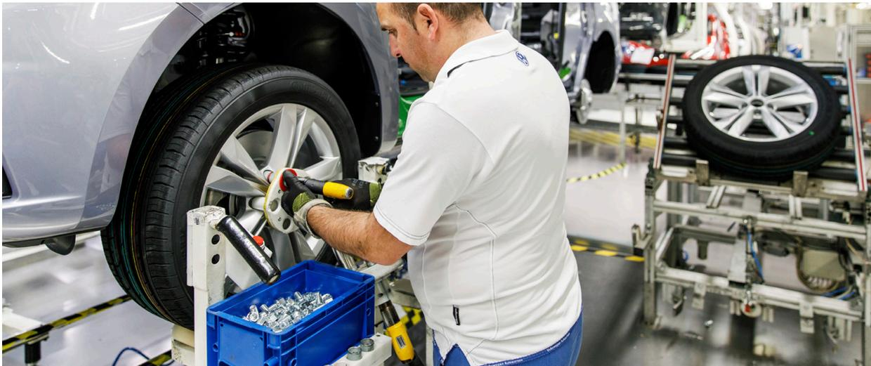
3D printed manufacturing aids are used by Volkswagen Autoeuropa to maximize production efficiency. For example, the pictured wheel protector jig prevents scratches and damage to wheel rims and simultaneously aligns an operator's pneumatic impact gun to speed up the fitting process and reduce scrap costs.
