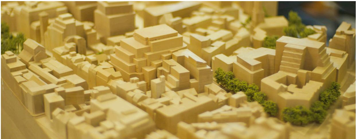
London-based MATT architects uses 3D printed concept models to communicate complicated ideas to their clients. Previously, they used hand-made paper or cardboard models. This was a labor-intensive and slow process that limited the range of ideas that could be conveyed. Now they can produce high-detail concepts within hours.
