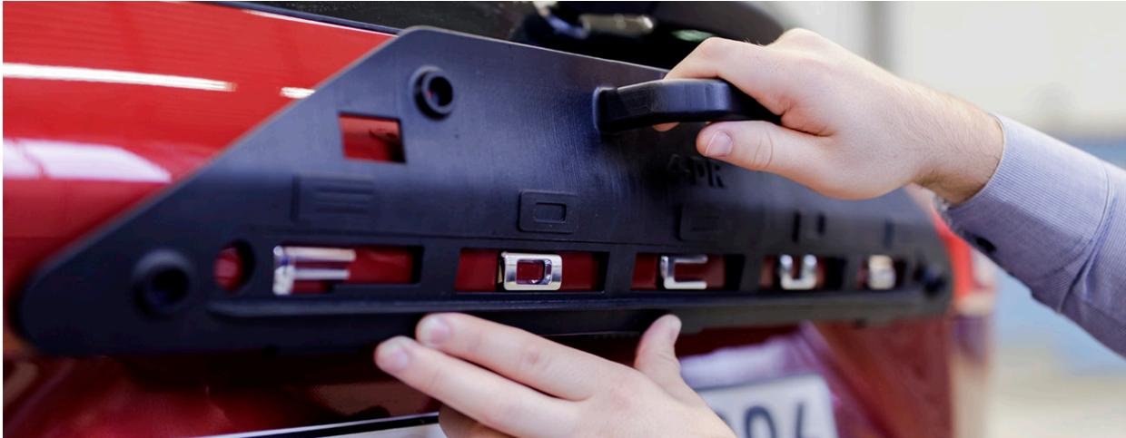
Ford Motor Company was able to implement more than 50 3D printed tools for high volume production of the All-New Focus, with considerable cost savings per tool compared to conventional methods. The alignment tool pictured above ensures that emblems and decals are consistent for each vehicle that rolls off the assembly line.
