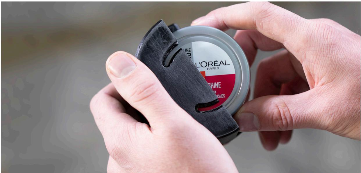
3D printed manufacturing aids make production easier, faster, and cheaper for world-leading beauty company L'Oréal. The pictured gauge keeps product packaging consistent by verifying that labels are correctly positioned. With standardized label placement and quality assurance, deviations are unlikely to hit the shelves.
