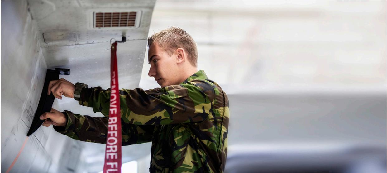
Performing maintenance on complex and customized aircraft can be an expensive challenge. By adopting 3D printing, The Royal Netherlands Air Force is able to affordably create tools for specific applications within hours. 3D printed parts cost approximately \$10 to produce, while traditional methods can cost over \$1,000 for the same part.
