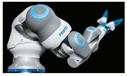
BionicCobot is a pneumatic development of the Bionic Learning Network. It is the result of a project which investigates what the production of the future can learn from nature.
