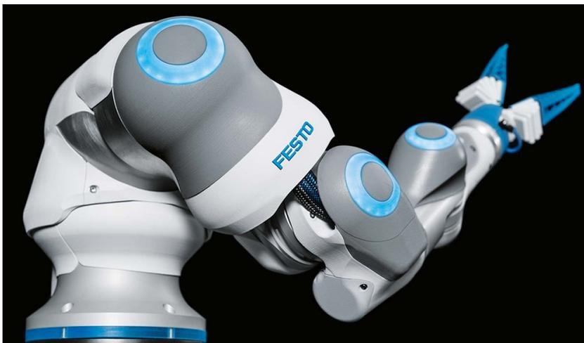
BionicCobot is a pneumatic development of the Bionic Learning Network. It is the result of a project which investigates what the production of the future can learn from nature.
