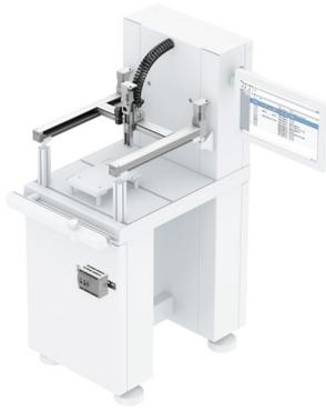
Small robots like a 2D or 3D gantry or cobot can be integrated into a functional work station with a minimal footprint to perform functions like testing or analysis or small parts handling. Such work stations can even be mobile, moved around a facility and plugged in wherever they are required.
